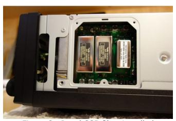
Figure 2. Inrad SSB filter installed
