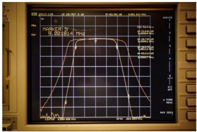
Inrad 2.1 kHz filter vs. Stock 3 kHz filter
